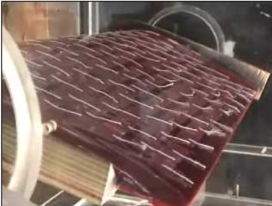
Figure 14: Tuft visualization test. From the image separation is evident from the tufts bending as the flow reverses direction. This is more apparent towards the centerline of the wing where the wind tunnel walls have no effect on the flow.
